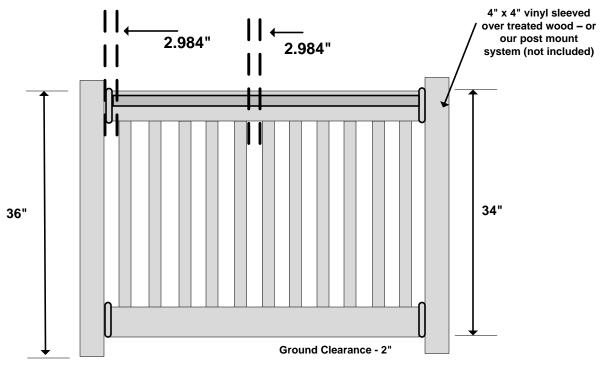
NOTE: No Aluminum in bottom rail. Foot Block is required for installation to meet the International Residential Code.
