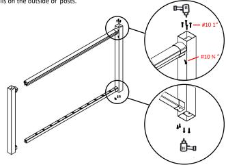
2. Install the pickets and spacers. Insert picket end into bottom rail and slide the opposite picket end into the top rail. Insert spacer for even pickets
