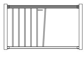
3. **Install the post caps.** Install and secure the caps with #10x3/4" pan head screws.
