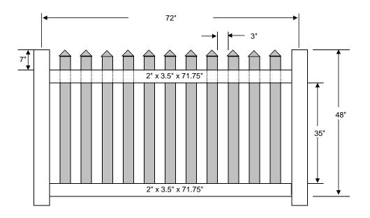
Panel can accommodate a slope of 7.5" over 6' using the racking method
