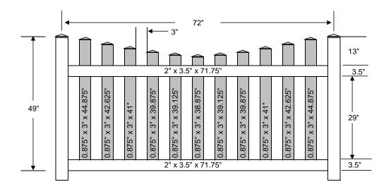
Panel can accommodate a slope of 7.5" over 6' using the racking method
