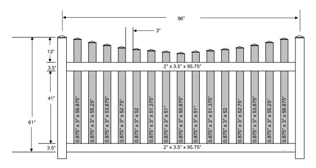
Panel can accommodate a slope of 10" over 8' using the racking method
