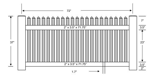
Panel can accommodate a slope of 6" over 6' using the racking method
