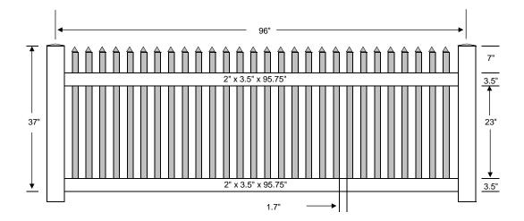
Panel can accommodate a slope of 8" over 8' using the racking method
