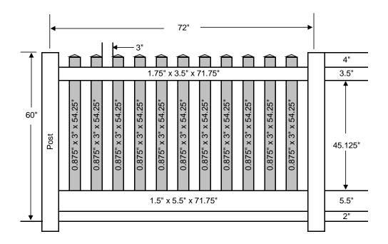
Panel can accommodate a slope of 7.5" over 6' using the racking method
