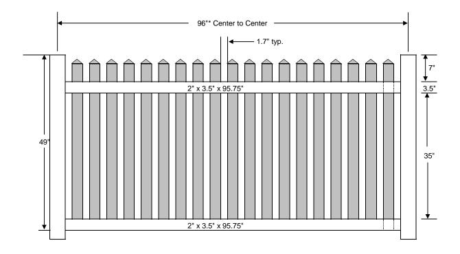
Panel can accommodate a slope of 8" over 8' using the racking method
