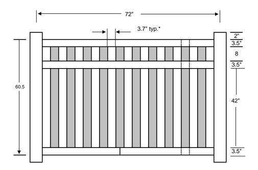
Panel can accommodate a slope of 4.5" over 6' using the racking method
