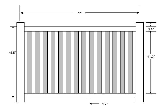
Panel can accommodate a slope of 6" over 6' using the racking method
