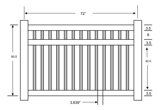
Panel can accommodate a slope of 4.5" over 6' using the racking method
