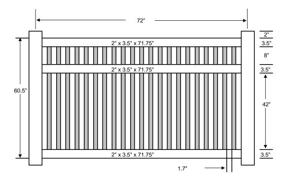
Panel can accommodate a slope of 3" over 6' using the racking method
