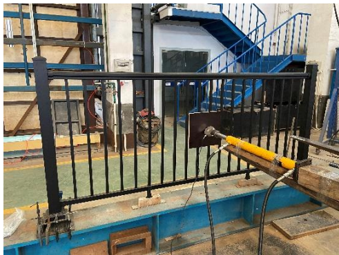
In-fill load position 1
