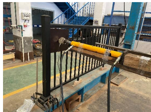
In-fill load position 2
