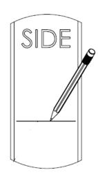
1. Make a straight, level line on the side of the gate at the desired height for the latch handle.
