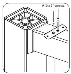
Insert a screw up through each of the 2 outer holes on the deck board clip securing the deck board into place.
