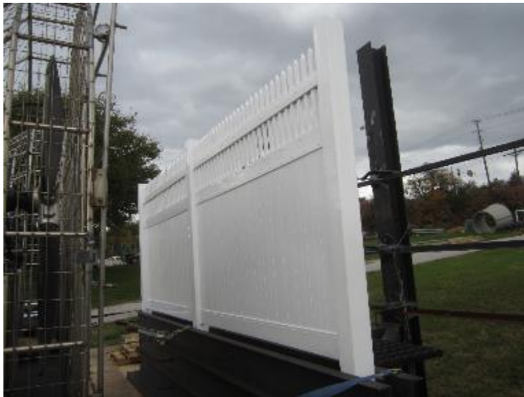
Photo No. 1 Wind Generator Outlet Relative to Test Specimen
