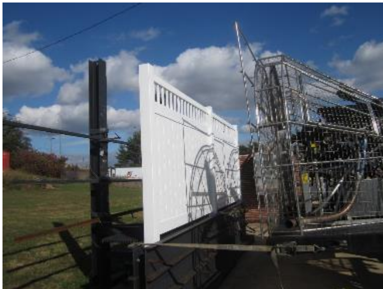
Photo No. 2 Typical Dynamic Wind Load Setup
