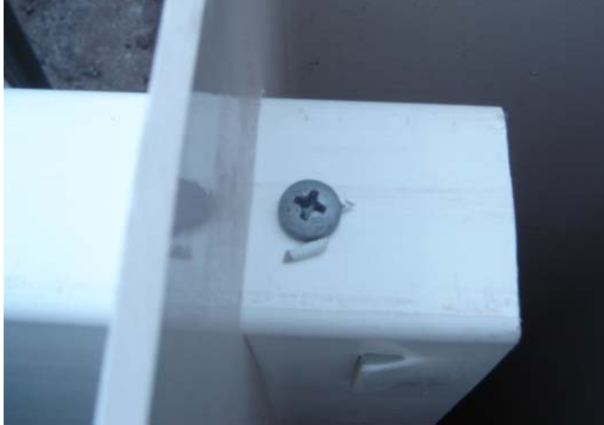
Photo No. 5 Test Specimen No. 2 and 4: #10 Screws in Top of Top Rail at Both Ends
