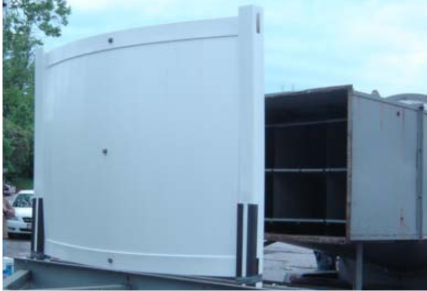
Photo No. 7 Test Specimen No. 3: Pembroke Less Mechanical Fasteners at 90 mph Wind Load
