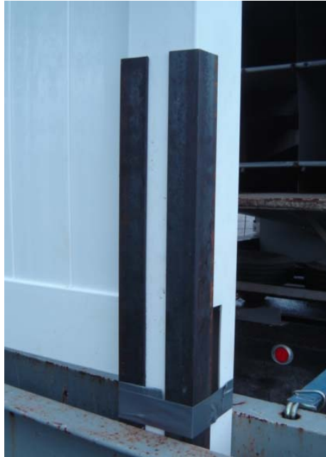
Photo No. 3 Typical Post Reinforcement during Dynamic Wind Load Testing
