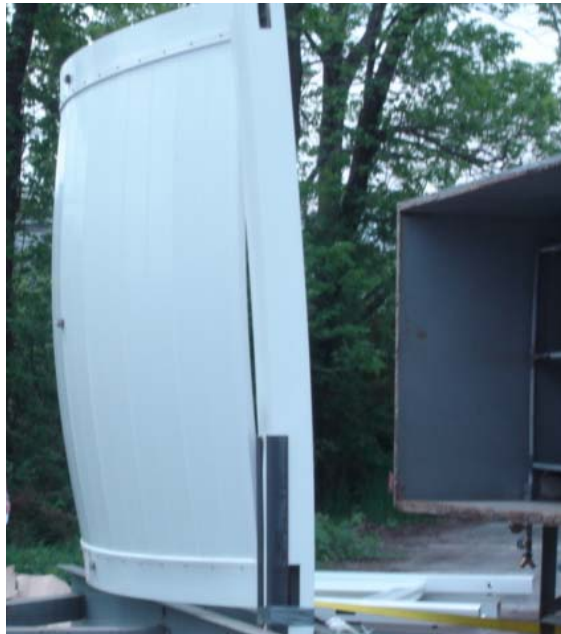
Photo No. 8 Test Specimen No. 4: Pembroke with Pickets Screwed to Rails at 110 mph Wind Load
