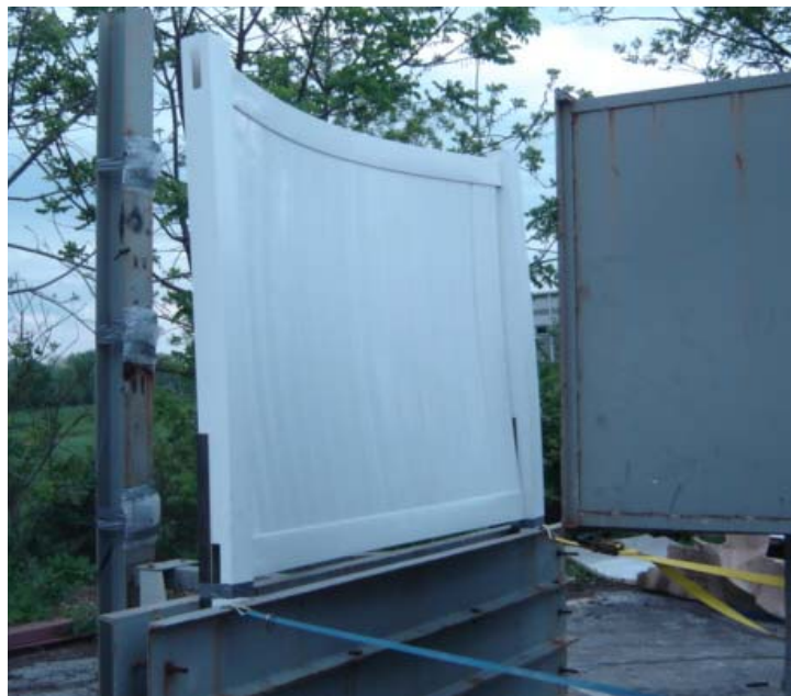
Photo No. 4 Test Specimen No. 1: Savannah Less Mechanical Fasteners at 90 mph Wind Load
