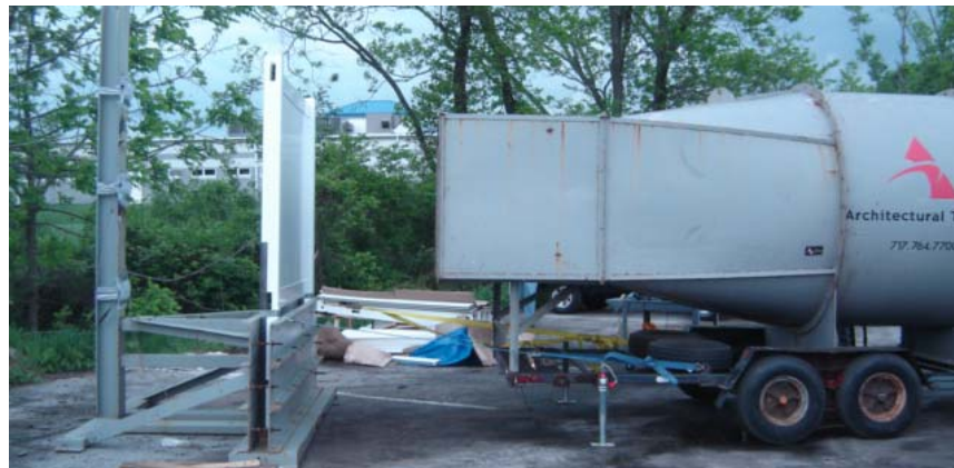
Photo No. 2 Test Specimen in Rigid Test Fixture 48 in from Wind Generator Outlet
