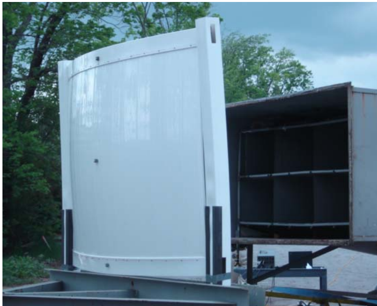
Photo No. 6 Test Specimen No. 2: Savannah with Pickets Screwed to Rails at 100 mph Wind Load
