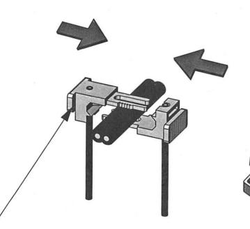
**Step 1** - Make the connection from the cap to the low voltage cable by placing the connectors on each side of the low voltage cable and pressing together until connectors are seated firmly together.
