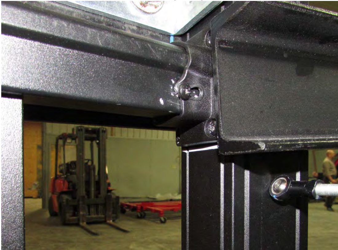
Test Sample #3 - Screw Pulling Through Bracket at 589 lbf.
