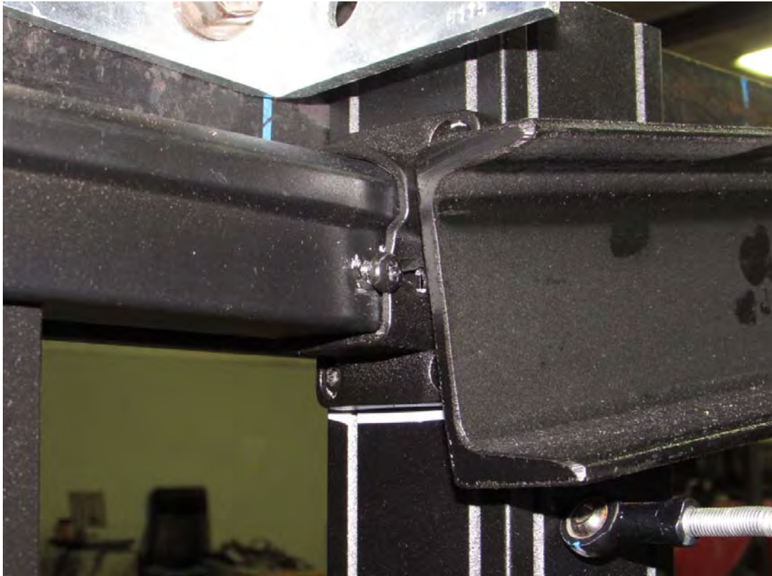
Test Sample #2 - Screw Pulling Through Bracket at 586 lbf.
