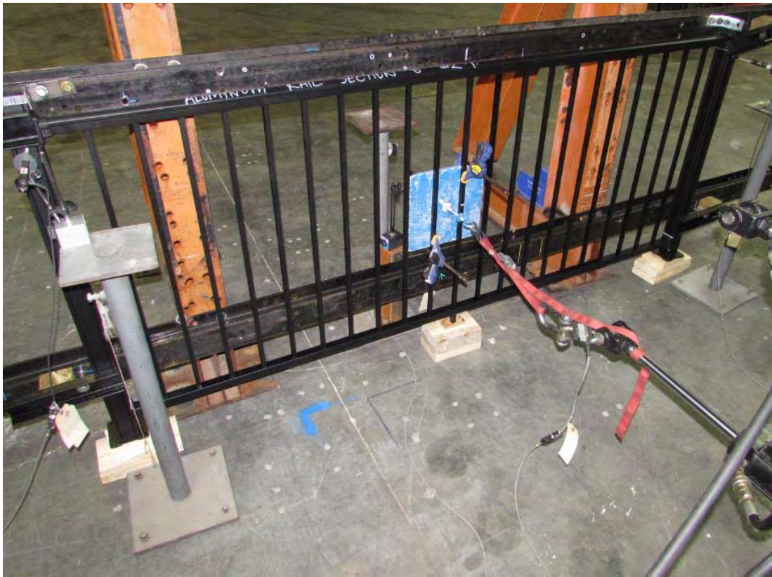
Typical In-fill Load Test Setup
