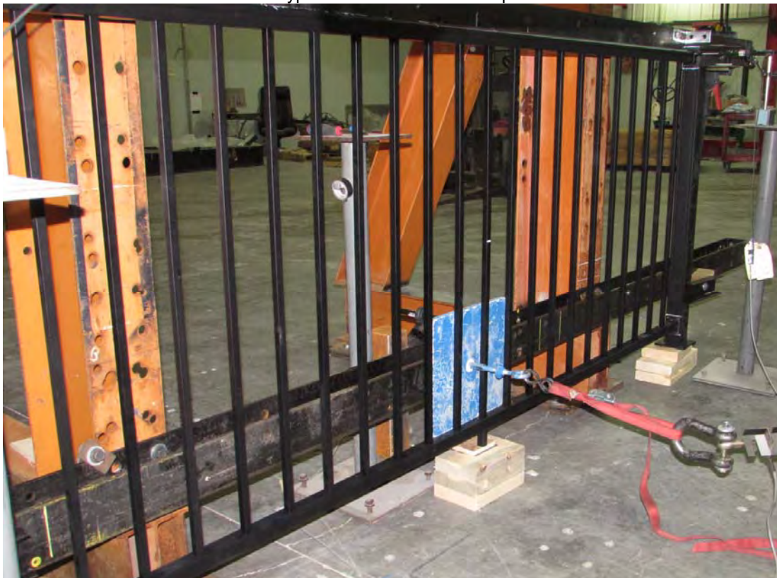
Typical In-fill Load at Bottom Rail Test Setup
